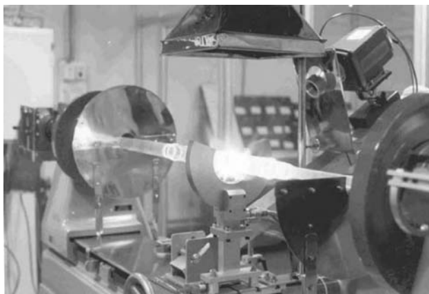
FIGURE 4.21 Preform fabrication setup. (Courtesy of Dr. S. K. Bhadra, CGCRI, Kolkata, India.)
